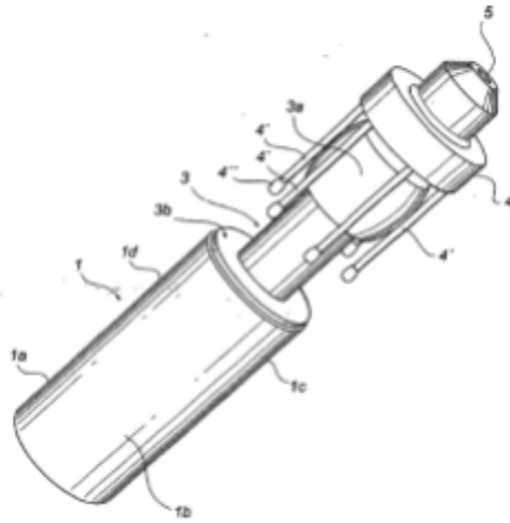
Figure 6. Micropositioning Device Patent. Image from Micropositioning device , by Olin, H., et. al., 2003 Patent.
